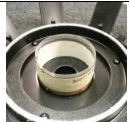
VC should fit snugly in gap w a few windings showing
